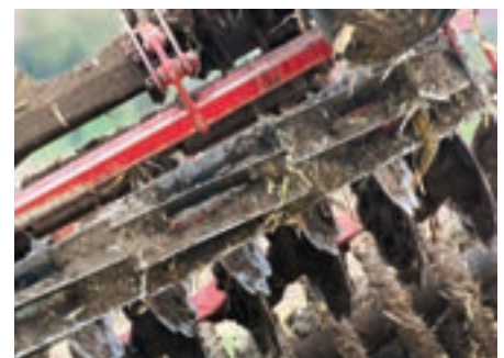
For the 5.75-meter wide Joker 6 RT the knife roller is divided into three segments
