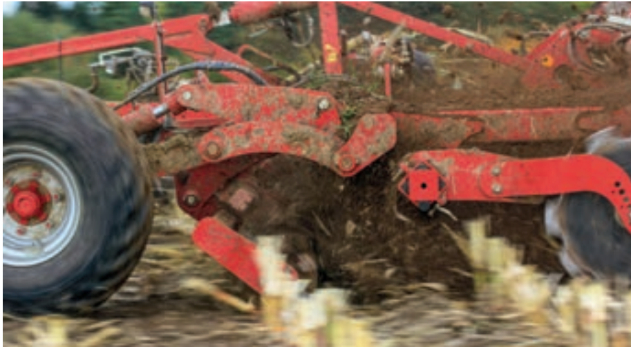
The knife roller works most efficiently at operational speeds between 15 and 20 km/h.
