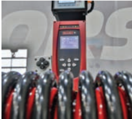
Automated assembly of a TerraGrip tine with torque safety system: only if the part meets the required quality standards (green tick – right photo), it will be installed in the machine.
