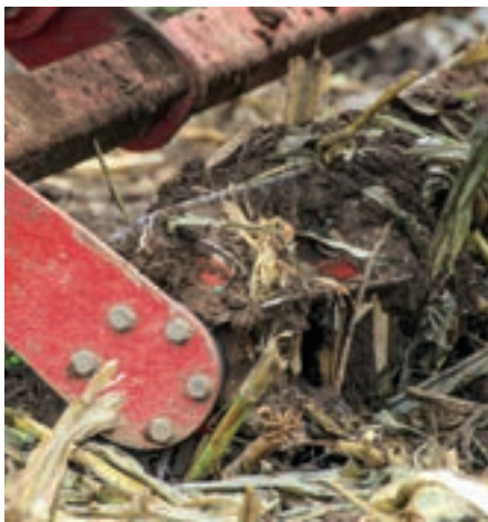
Self-cleaning: On cohesive soils harvest residues and soil can adhere to the knives. However, you can still go on working.
