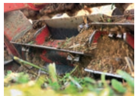
The six self-sharpening knives are screwed in a slightly diagonal way to a closed shaft – thus a high cutting pressure is possible.
