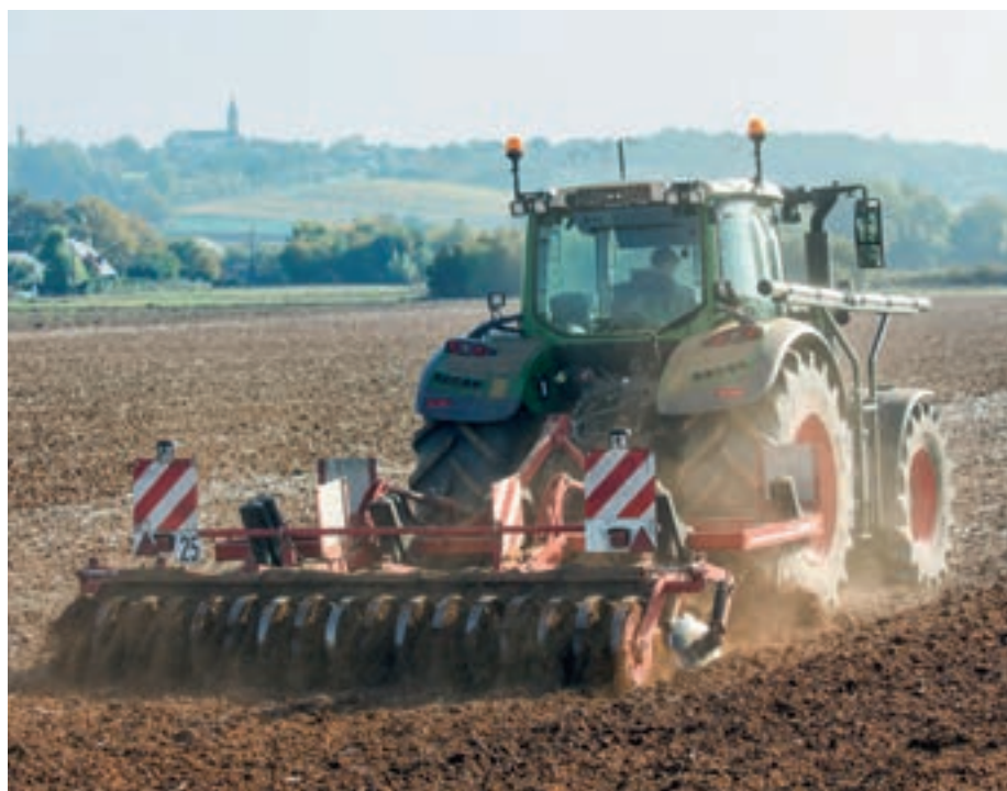
The Terrano FX is used before sowing. It is equipped with MulchMix points, penetrates the soil excellently, cuts it open and allows for an optimum mixing of soil and straw.
