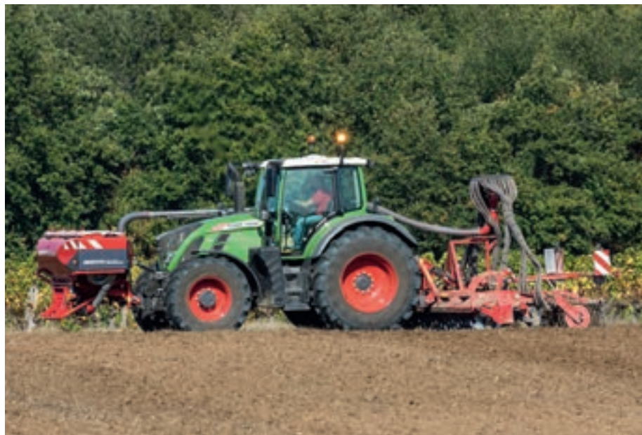
For sowing wheat, the farmer uses a Joker CT in combination with a Partner FT to avoid compactions and to save one pass.
