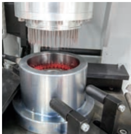
The needles fill the bearing with exactly the required quantity of grease (left photo). The subsequent fitting of the bearing stub is documented accurately (right photo).
