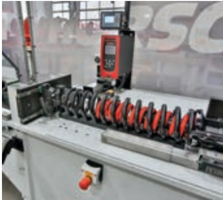
Automated assembly of a TerraGrip tine with torque safety system: only if the part meets the required quality standards (green tick – right photo), it will be installed in the machine.
